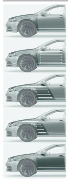
Adjacent panel: sand panel with suitable abrasive e.g. Trizact - P1000 New part / repair: sand surfacer (minimum P500)
