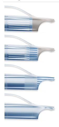
Apply Standoblue Color Blend / Color Blend Slow\* to the surrounding fade out area or adjacent panels with thin closed coats.
