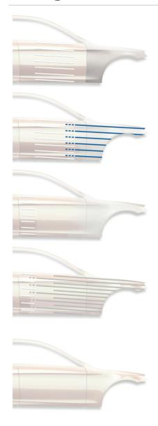
Apply a closed coat of hardened Standoblue Color Blend / Color Blend Slow (blender +10% Standoblue Hardener) to the adjacent blending areas, avoiding the extreme edges of the panel.
